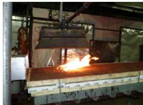
Test facility approx. one minute after the two incendiary agents were put in place, fuelled by the airflow from the blower.
