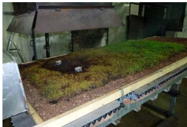
The 30 minute radiant heat led to the vegetation drying out across a diameter of about 80 cm
