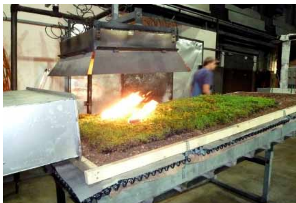
Testing equipment for test procedure 3 with a vegetation mat in place
